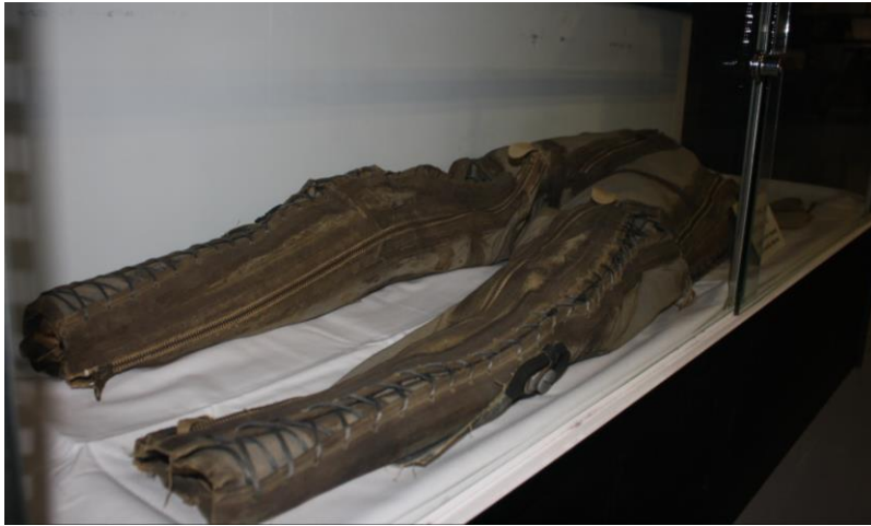
Frank Anti-Gravity Flying Suit Water Filled Mk III Developed by Dr Wilber R. Franks Institute of Aviation Medicine
